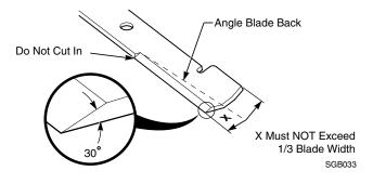
Figure 7-7. Blade Sharpening
